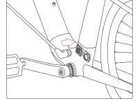
2. Connect the DC output plug from the charger to the charging port.
