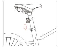
2. Slide the seatpost in or out of the seat tube.
