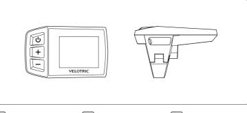
Ung press for 2 seconds : • Power on/off Single press: • Switch riding data
