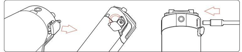
5. Plug the charger into a power outlet to initiate the charging. It may take about 6 hours for an empty battery (battery level 0%) to be fully charged. You can check the charging status through the indicator on the charger. For more information, refer to "[Charger Indicator Status](#)".
