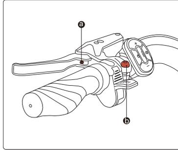
If you have big/small hands or find it difficult to squeeze the brake levers, you can also adjust the distance between the brake lever and the handlebar according to the steps below.
