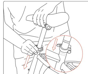
3. Align the seatpost clamp opening with the notch in the seat tube, and close the seatpost clamp lever fully.
