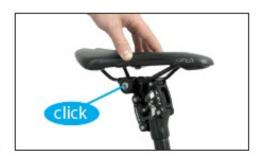
4. Adjust the saddle so that it is centered and the top surface to be horizontal (recommended) as shown in the picture on the right.
