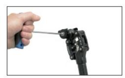
2. Install the saddle by inserting the rail into the clamp from one side.
