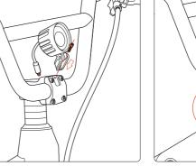
Install the display onto the handlebar, adjust it to an angle you can view easily on the seat
