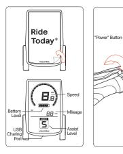
Assist level 1 Eco Mode: Minimal power output for maximum battery efficiency.
