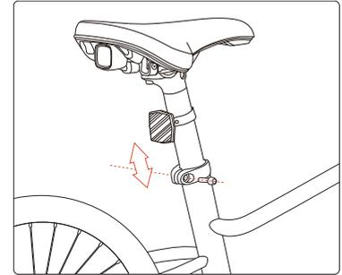
3. Tighten the seatpost clamp with an M5 Allen key. Ensure that the clamp is firmly tightened.
