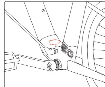
2. Connect the DC output plug from the charger to the charging port.
