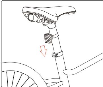
2. Slide the seatpost in or out of the seat tube.
